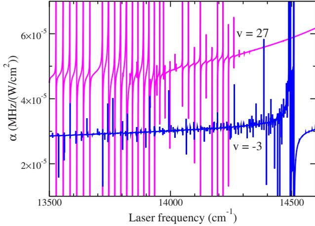
FIG. 8. (Color online) Real part of the dynamic polarizability of the  $J=0$  vibrational levels of the  $\text{Sr}_2 X^1\Sigma_g^+$  state as a function of laser frequency in the range of 13 500–14 600  $\text{cm}^{-1}$ . For clarity, only two selected vibrational levels of the  $X$  state are shown,  $v = -3$  and  $v = 27$ . The polarizabilities are evaluated at 0.1- $\text{cm}^{-1}$  intervals. The polarizabilities of  $J=0$  rotational levels are independent of the laser polarization.
