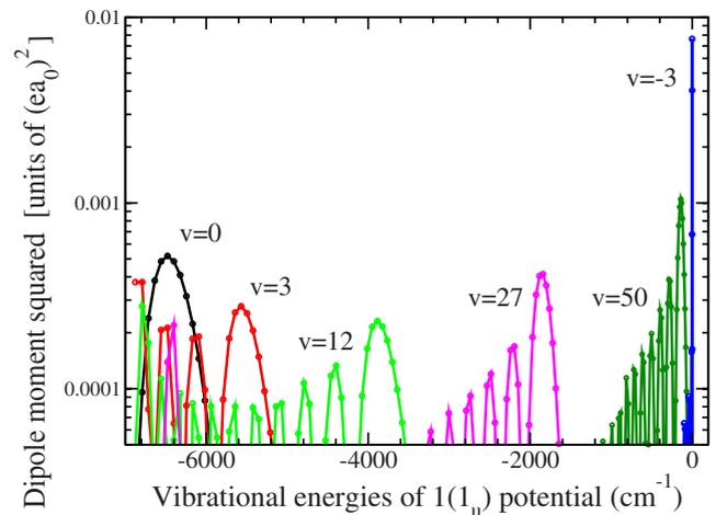
FIG. 3. (Color online) The square of the vibrationally averaged dipole moments for transitions from selected vibrational levels (all with  $J=0$ ) of the  $X^1\Sigma^+$  electronic ground state as a function of the energy of vibrational levels (with  $J'=1$ ) of the  $1(1_u)$  potential of Sr<sub>2</sub>. Each curve corresponds to a single rovibrational level of the  $X^1\Sigma^+$  state. Zero energy corresponds to the  $^1S_0+^3P_1$  dissociation limit.
