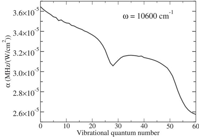
FIG. 6. Real part of the dynamic polarizability  $\alpha$  of the  $J=0$  levels of the  $X^1\Sigma^+$  ground state of  $\text{Sr}_2$  as a function of vibrational quantum number for infrared laser frequency of  $10\,600\text{ cm}^{-1}$ .
