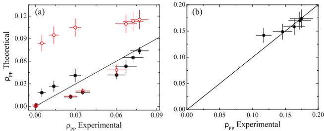
FIG. 2 (color online). Panel (a): experimentally determined excitation fraction in  $Ba^+$  versus theoretical predictions of the quantum Liouville (●) and rate equation (○) treatment. Panel (b): experimentally determined excitation fraction in Ca versus predictions of a 4-level rate equation model. In both panels the solid line has a unit slope, representing ideal agreement.
